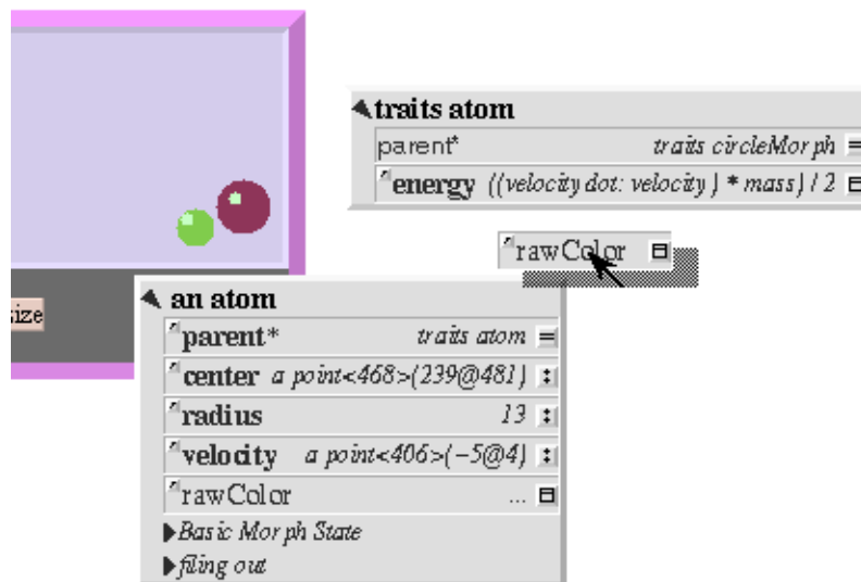
Figure 10. The user copies the modified rawColor slot as a first step in getting the computed method of coloring more widely shared. Because slots can be moved about readily, restructuring changes are relatively light weight, enhancing the sense of flexibility.
