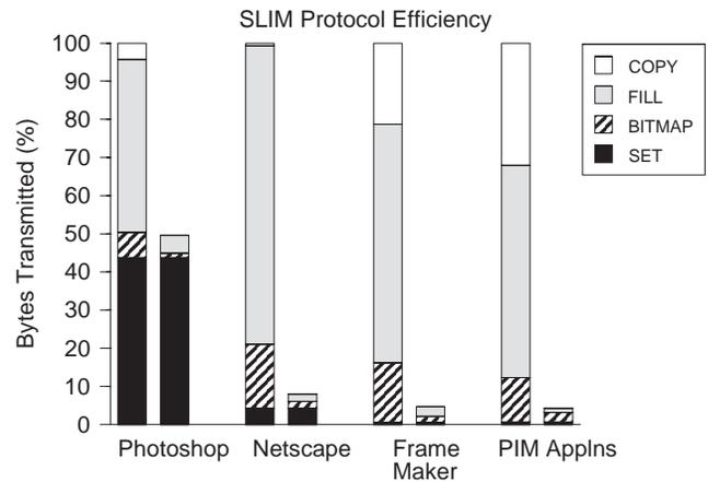
**Figure 4** Efficiency of SLIM protocol display commands. The left-hand bar in each set depicts uncompressed data, and the right-hand bar depicts use of the SLIM protocol. CSCS is not used in these benchmark applications.
