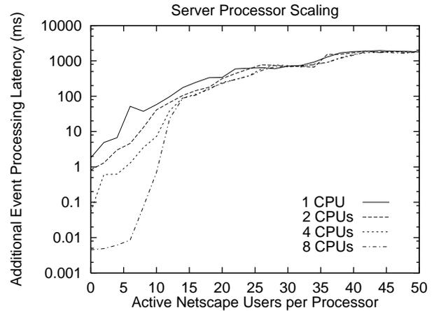
**Figure 10** Average latency added to 30ms processing time for events occurring at 150ms intervals as the number of active Netscape users increases (1-8 active CPU’s). User processor loads are generated with a trace-driven simulator which “plays back” previously recorded resource usage profiles.
