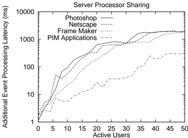
**Figure 9** Average latency added to 30ms processing time for events occurring at 150ms intervals as the number of active users increases (1 active CPU). User processor loads are generated with a trace-driven simulator which “plays back” previously recorded resource usage profiles.
