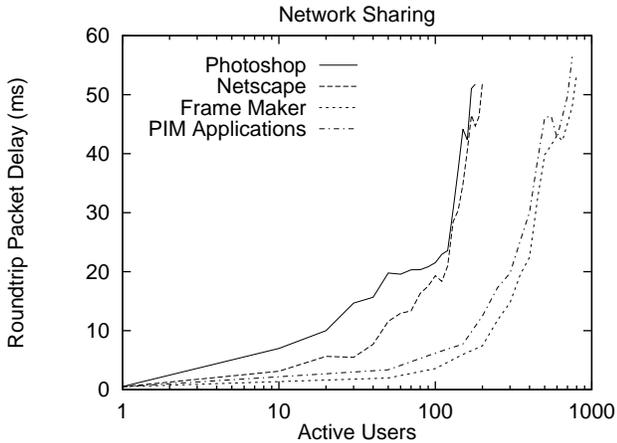
**Figure 11** Network round-trip latency for 64B upstream packet followed by 1200B downstream packet. User traffic loads are generated with a trace-driven simulator which “plays back” previously recorded resource usage profiles.
