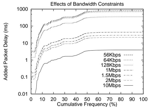
**Figure 6** Cumulative distributions of added packet delays for Netscape traces of SLIM protocol commands captured at 100Mbps and retransmitted on simulated networks with lower bandwidths. Bandwidth is averaged over 50ms intervals, and the histogram bucket size is 0.01ms.
