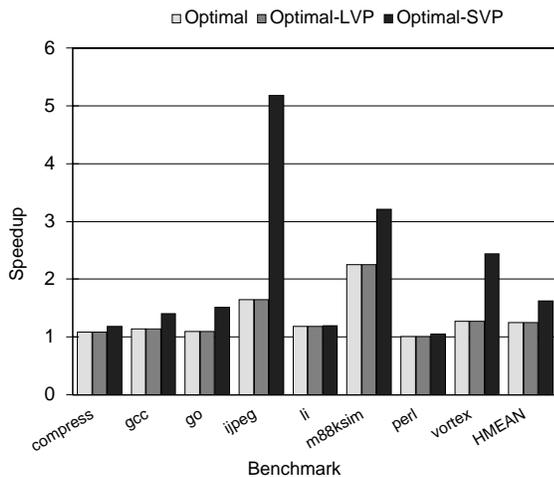
Figure 2. Optimal STP Speculation on Single-Level Loops
