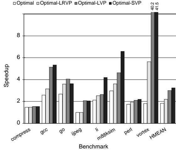
Figure 5. Optimal STP Speculation on Procedures
