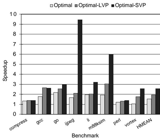
Figure 3. Optimal STP Speculation on Multi-Level Loops
